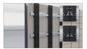
Fasten Omega profile with Al blind rivet (Art. no. 658) or A4 stainless steel screw (Art. no. 659) (Pay attention to fixed and sliding point)
