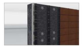
Click in the joint profile (for closed joints)
