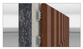
Securing of the position of the panels at the K20 Omega profiles (with securing brackets)
