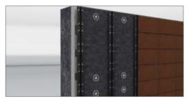
Mount the T-profile with approved fastening means
