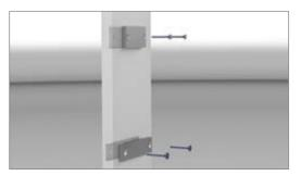
Fix base plate at the basic substructure
