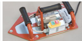
TILE VIBRATOR OR RUBBER ANTI-BOUNCE BEATER.
