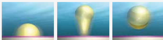
Oil and grease detach from the surface.
